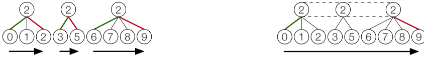
(a) Separate iterators over the duplicates' children. (b) Chained iterator over the duplicates' children.
