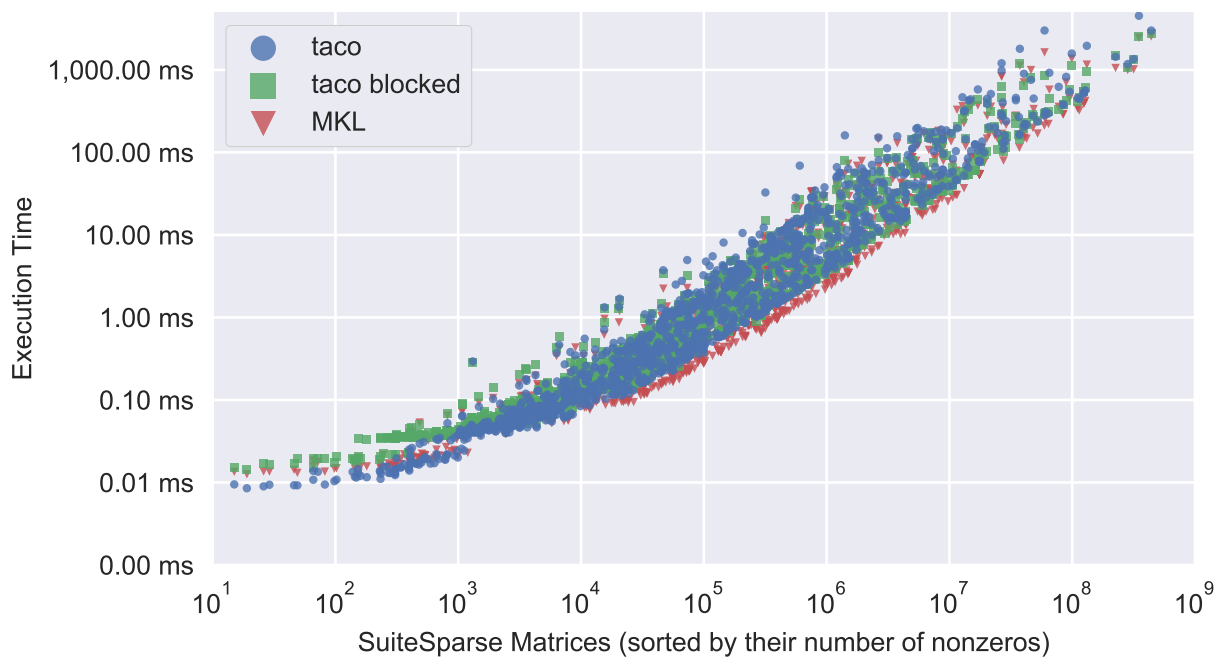
Figure 7-11: SpMM CPU with the CSR format
