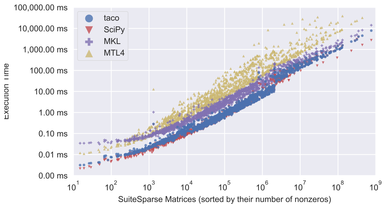
Figure 7-15: Matrix Addition CPU with the CSR format.
