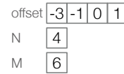
Figure 2-19: Range data structure. Each segment is stored as range offsets and sizes.
